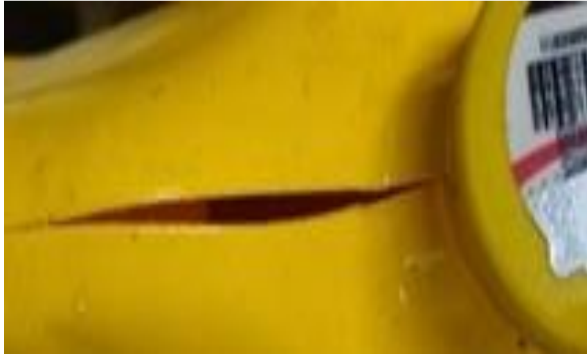
Gambar 3.16 Cacat Seam Split
